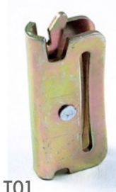
LT01 SPRING FITTING, 4500LBS FINISH: YELLOW ZINC PLATE
